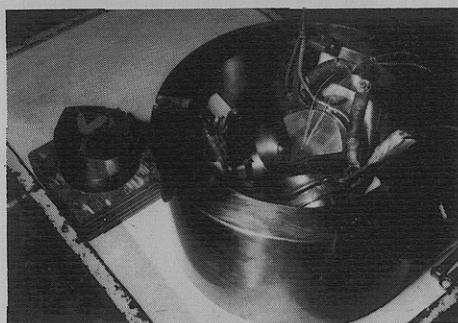
Figure 3. Photograph of the central part of the tetrahedral anvil high-pressure apparatus.
